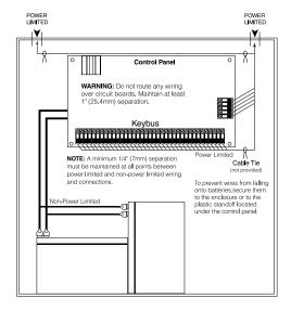
**NOTE:** Wire entry for power limited wiring must be separated by a different entry access from non-power limited wiring.
